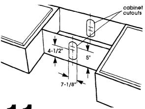
To vent through the roof with 7" round ductwork, mark 4-1/2" and 5" in from back wall along the centerline on underside of cabinet. Use these points as centers to draw 7-1/8" circles on underside of cabinet. Use a saber saw to cut the openings for the ductwork. Repeat for the underside of the top of the cabinet. This will create slotted openings.
